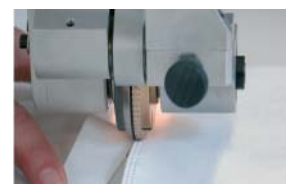
PFAFF 83 12 CS One wheel solution-machine - flatbed-version = cut edge and welded
