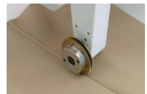
PFAFF 83 10 CS dual New double wheel solution - flatbed-version = simultaneous cutting and welding
