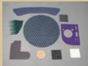
TexCut 3001 cutting pattern: floor covering for aircraft, glassfiber material (GFK), fitted carpet, conveyor belt, industrial textile, soft-top/tilt fabric.
