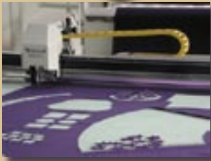
TexCut 3001 for the processing of single layers of industrial fabric.
