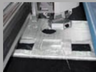
Multi-layer fabric fibers during processing on the TexCut 3070 (Figs. top and bottom).
